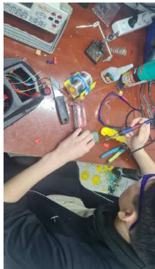
Figure 3 – The process of soldering and designing the controller
